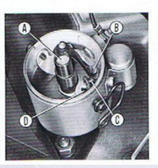
To adjust the gap slacken screw B, insert a screwdriver in slot D and turn the fixed contact plate as necessary. Retighten the screw.
