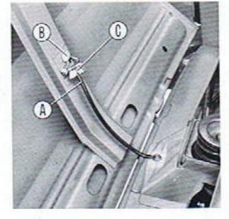
Mount the spare wheel ensuring that the peg fits in one of the associated holes in the wheel disc.
