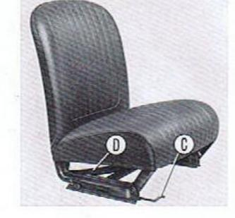
Ensure that the lever engages the nearest locking notch.
