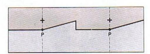
Note: The beam pattern shown applies to R.H. traffic countries. A reversed beam pattern should be obtained on cars operating in L. H. traffic countries.
