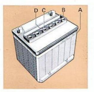
Note: The shape of well B may vary according to battery manufacturer.
